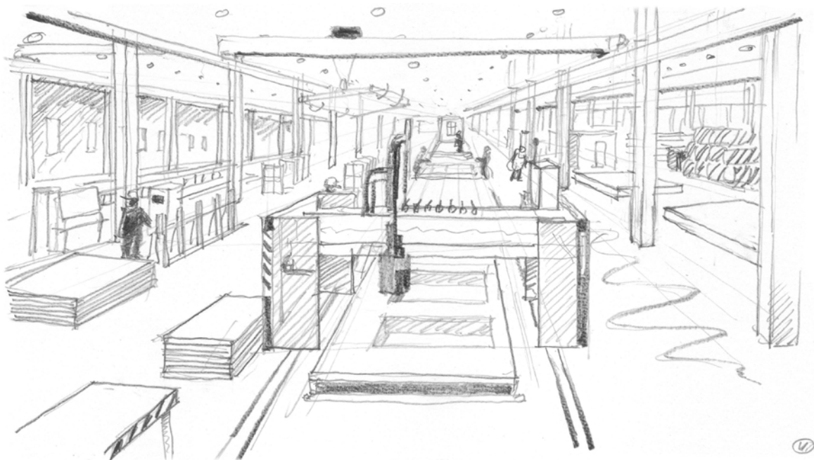
10. Hoone elemendid toodetakse tehases ning monteeritakse ruumilisteks mooduliteks The building elements are produced in the factory and assembled into modules
